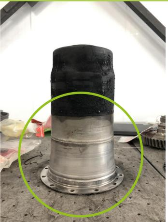
P&W shaft housing Soaking for 7 minutes in an ultrasonic basin and rinsing with water.
