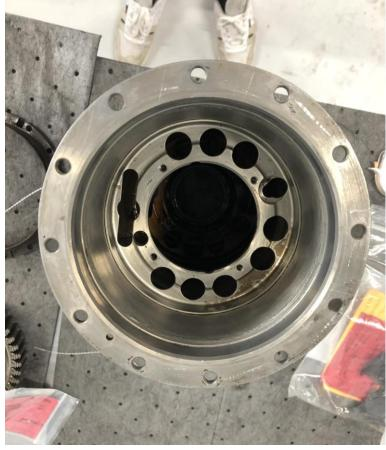
Carter d'arbre P&W Soaking for 7 minutes in an ultrasonic basin and rinsing with water.
