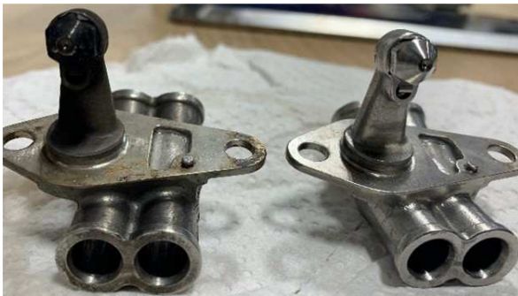
On the right, fuel injector nozzle for P&WC turbine engine after 5 minutes soaking in using an ultrasonic basin. The hardened carbon is completely removed without having to disassemble the part. See next page for other before/after examples.
